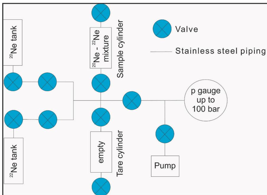
**Fig. 1.** Schematics of the apparatus used to prepare the artificial gas mixture of  $^{22}\text{Ne}$  and  $^{20}\text{Ne}$  at KRISS. At each step of the fill (empty,  $^{22}\text{Ne}$  charge and  $^{20}\text{Ne}$  charge), the mass of the sample cylinder was compared to that of tare cylinder using a Mettler Toledo model AX1005 precision electronic mass comparator.
